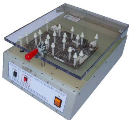
Figure 2: PCB Bed-of-Nails Test Fixture
